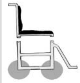
Seat frame independently mounted onto the wheelchair frame
