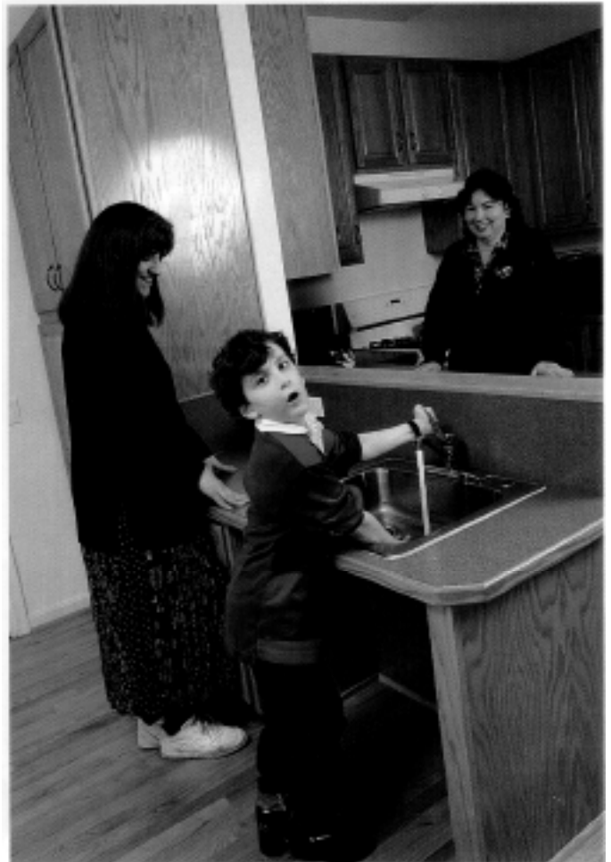
Jason has his own sink and countertop in the kitchen. The area under the sink is open so Jason can access the sink while in his wheelchair.
